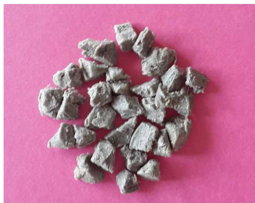
Figure 1. HDPE/cenosphere blend from brabender. [Color figure can be viewed in the online issue, which is available at wileyonlinelibrary.com .]
